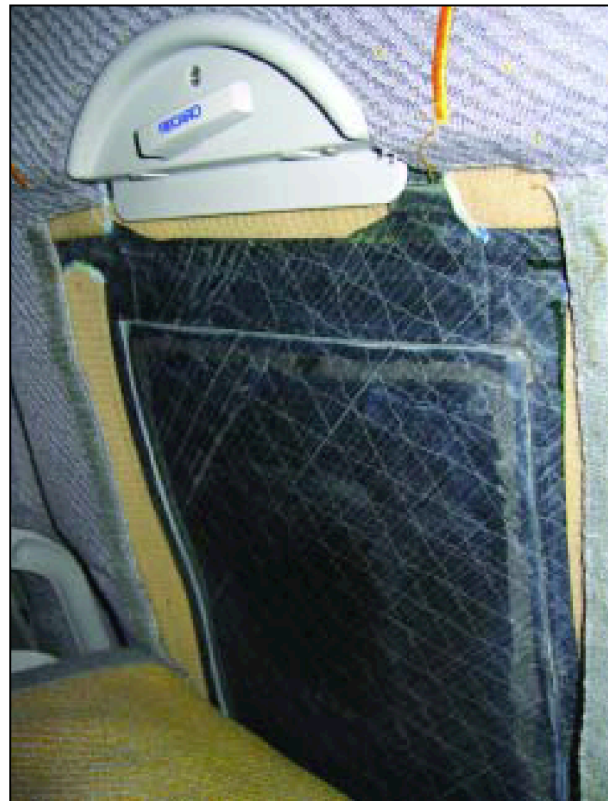
Applications for Bafatex's scrims include aircraft seating where, in this case, the polyester filament scrim is combined with a unidirectional carbon prepreg.
